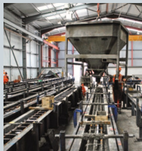
PRECAST PILING AND BEAM MANUFACTURING
